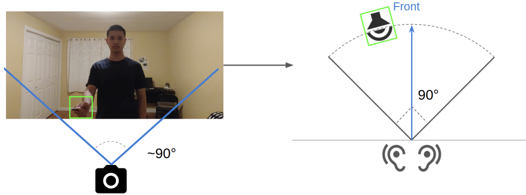
Figure 10. Illustration of the Audi-Exchange Experiment. The hand-tracking and 3D audio algorithms translate visual interaction cues of an extended hand into a 3D audio signal for the BVI user. Camera image shown was cropped to better fit the page. “Camera”, “speaker”, and “ear” icons credit to Google
